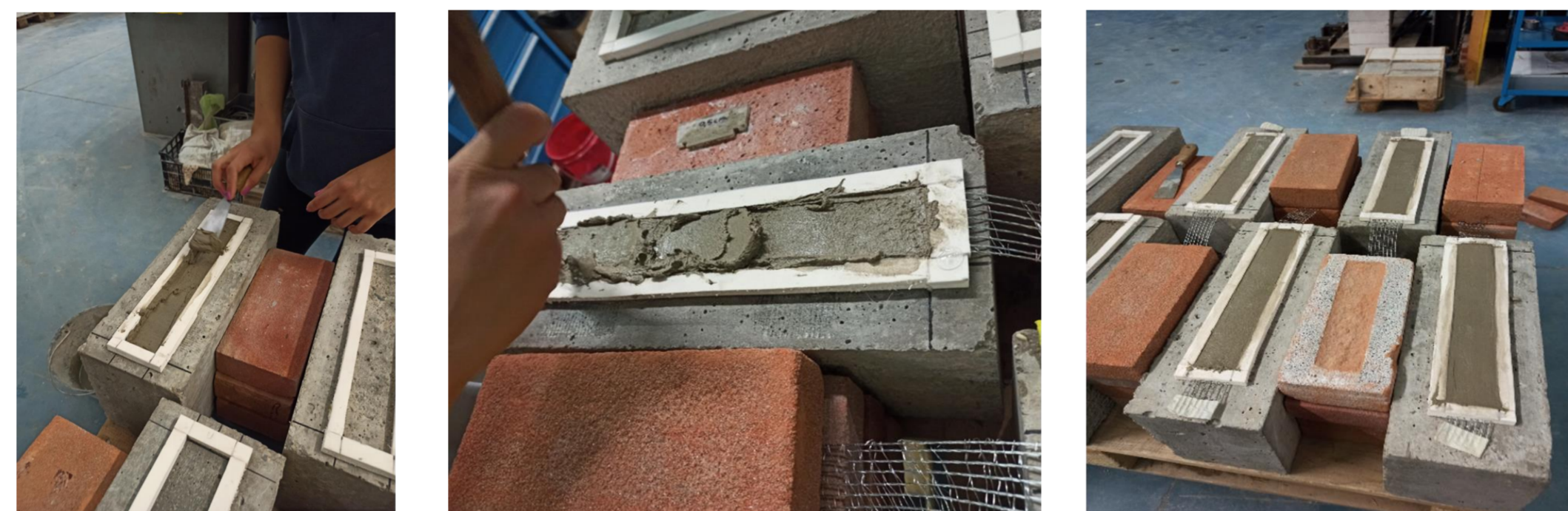
Specimen preparation with concrete substrate and reinforcement system made of GLV steel fabrics and cementitious mortar
