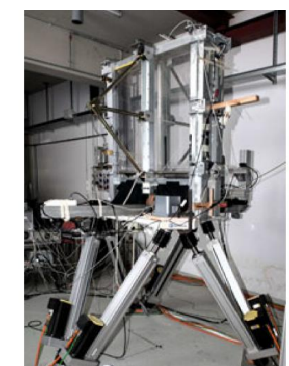
Figure 13 – Sloshing mechanism of the CNR-INM Sloshing Lab
